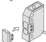
※ Both a slit and a filter can be used simultaneously.
