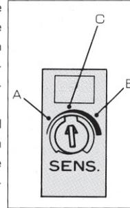
3. Point C midway between A and B is the optimum sensitivity position.
