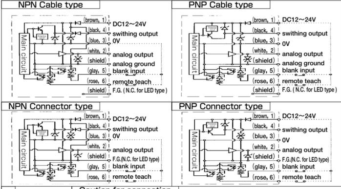
1) Connect the lead wires correctly. The analog output wire must not be in contact with any other wire. Do not turn on any power while wiring.
