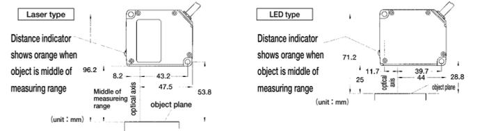
Note : ○ Adjust the sensor position so that the optical plane of the sensor is parallel with the plane of the object to be detected to obtain reliable measurement.
