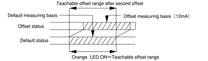
· Note : ○In default status, the sensor has been offset using white alumina ceramic. If not necessary to offset, you can skip this step.
